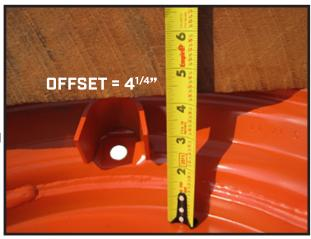
The terms **Inset** and **Outset** are used to describe how much a wheel mounting surface differs from the centerline of the skid steel wheel.
