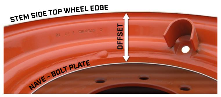
To help determine you **skid steer wheel offset** we put together a quick guide on how to accurately determine your wheel offset before purchasing. It's easy to assume that all skid steer wheels have the same nave plate (bolt plate) depth as the other, but unfortunately this is not always true. Although some skid steer machines share a standard size wheel, it;s best to measure this for ourselves to assure that we are providing you with a wheel that is designed for your machine.
